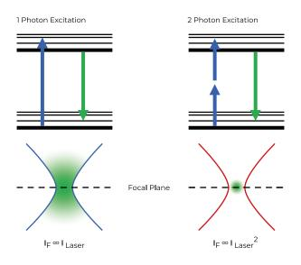
FIGURE 1. One-photon vs Two-photon Excitation.
